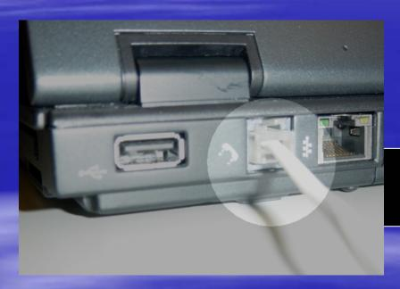
1. Plug the modem cable into the modem connector.
