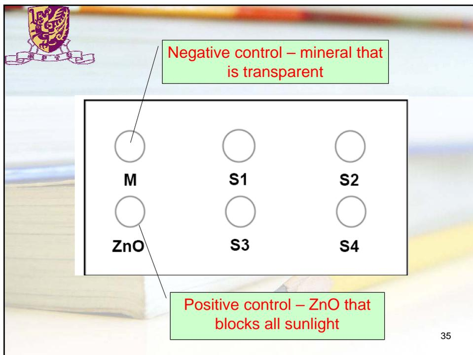
The diagram shows a 2x3 grid of experimental conditions. The top row contains conditions M, S1, and S2. The bottom row contains conditions ZnO, S3, and S4. Each condition is represented by a circle with its label below it. A callout box points to the M condition, stating: "Negative control – mineral that is transparent". Another callout box points to the ZnO condition, stating: "Positive control – ZnO that blocks all sunlight".
